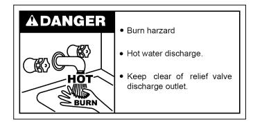
When checking the temperature-pressure relief valve operation, make sure that (1) no one is in front of or around the outlet of the temperature-pressure relief valve discharge line, and (2) that the water discharge will not cause any property damage, as the water may be extremely hot. See Figure 30.
